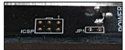
Important!, if the ICSP header is loose in the Pcb then hold it to one side so that all 6 contacts are made.
