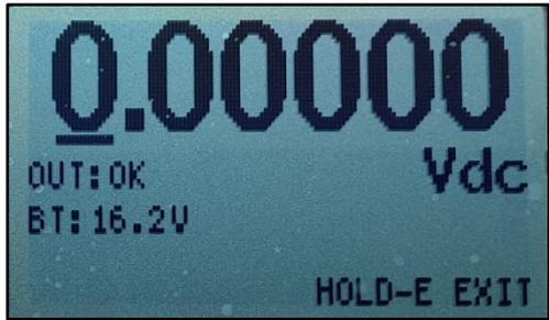
Initialize: The splash screen is displayed on power up with the software version before displaying the MAIN screen. It is recommended to wait 10mins from cold to allow the LM399AH reference to stabilize.
