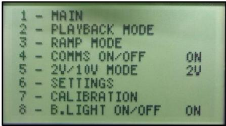
Initialize: The splash screen will be displayed on power up displaying the software version before displaying the MAIN MENU. It is recommended to wait 10mins from cold to allow the LM399AH reference to stabilize.
