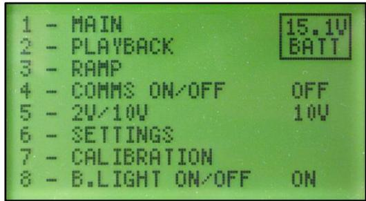
Initialize: The splash screen is displayed on power up with the software version before displaying the MAIN MENU. It is recommended to wait 10mins from cold to allow the LM399AH reference to stabilize.
